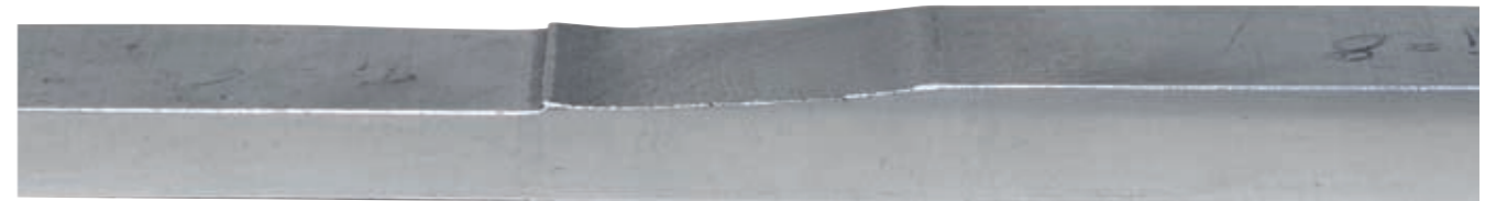
Figure 31. Tailor-welded blank on AA5754 H22, employing thicknesses 1 and 2 mm. Welding was carried out using a fixture featuring an inclined table at a speed of 6 m/min. © ESAB
