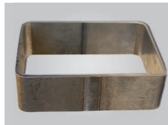
Figure 27. A longitudinal FSW weld in a rectangular profile. Beams can be manufactured with minimal distortion.
