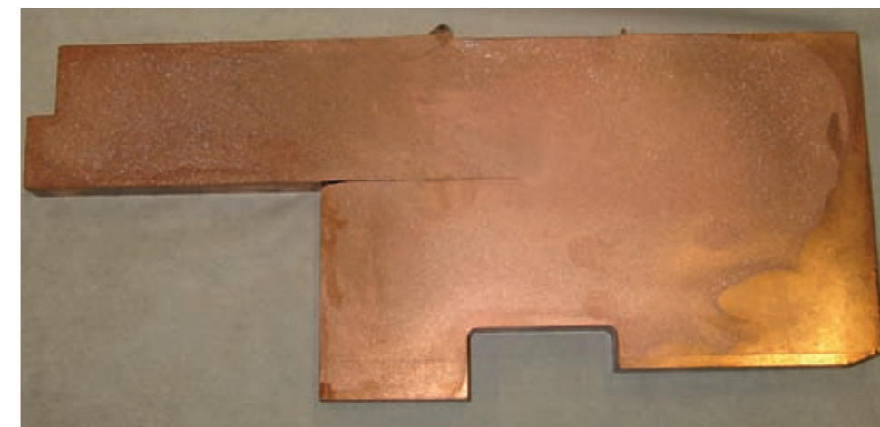
Figure 41. Cross section area of the FSW welded lid for the copper canister with a corrosion barrier thickness of 5 cm.
