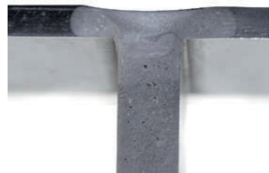
Figure 23. Etched microstructure on cast aluminium T-joint shows that the weld area has fine-grained microstructure without porosity. The fine "crack-shaped-line" coming from the right indicates a poorly stirred oxide-layer, not a crack.
