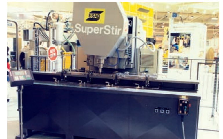
Figure 13. SuperStir™ #1 - first friction stir welding machine introduced to general public 1997 at the Schweissen & Schneiden Fair. Currently used at Boeing laboratories for research and development work.
