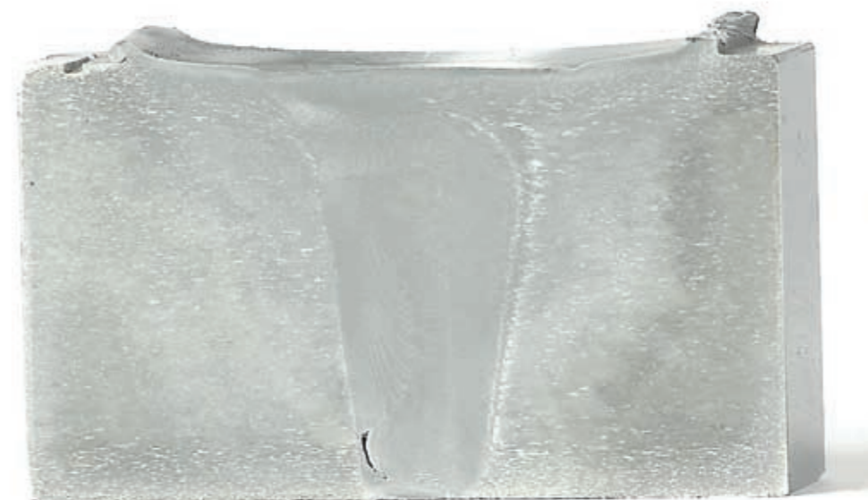
Figure 8. Etched microstructure of AA6082 welded with inadequate “heat input” in the root of the joint.
