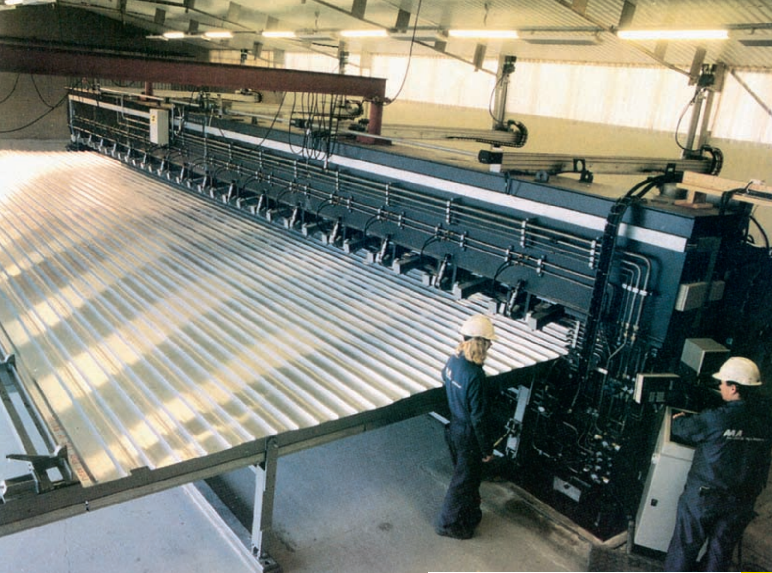
Figure 43. ESAB SuperStir™ FSW equipment installed at Marine Aluminium for welding panels.
