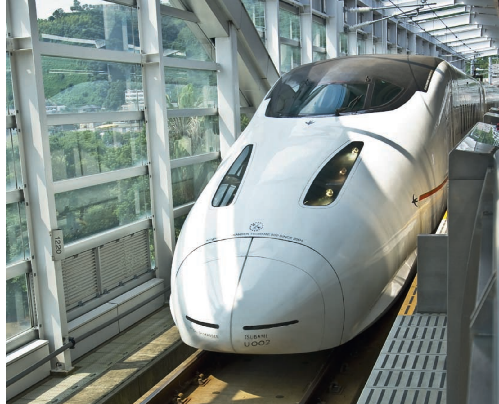
Figure 36. Shinkansen train. Friction stir welding is employed for the floor panels.
