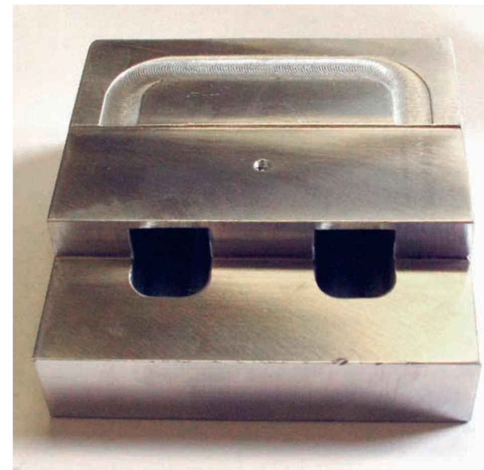
Figure 32. Machined heat zinc for electrical components to be used for e.g. automotive applications.
