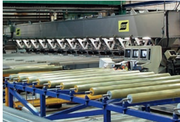
Figure 34. Fully automatic panel welding equipment at SAPA, Sweden. The equipment features three welding heads – two on the upper side, one on the lower side.
