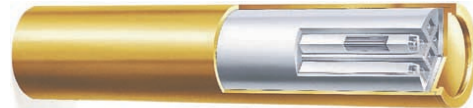
Figure 40. Copper canister with cast iron insert for nuclear fuel produced at SKB, featuring a lid sealed using ESAB Friction Stir Welding SuperStir™ equipment.
