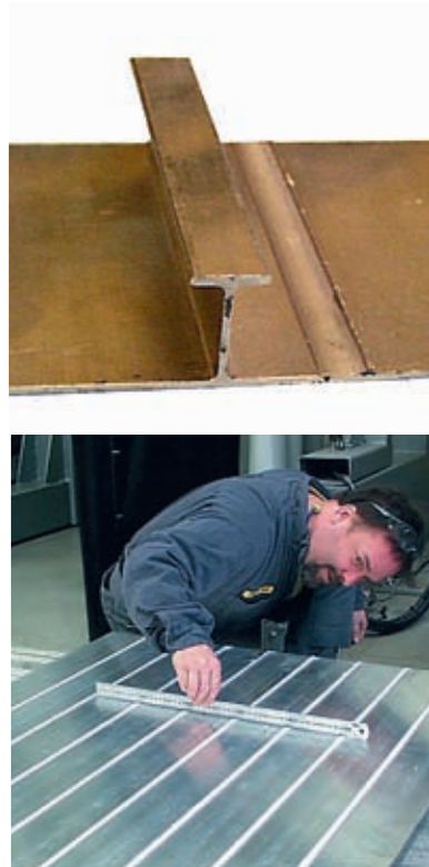
Figure 18. Flat panel field after welding. Instead of using wide profiles, the panel is made from relatively narrow (120 mm) extrusions. ©ESAB
