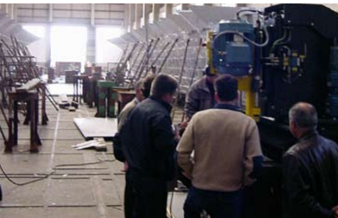
Figure 20. FSW LEGIO™ 3UT installed next to the aluminium ship hull production line at Estaleiros Navais do Mondego S.A. shipyard in Portugal, 2002.
