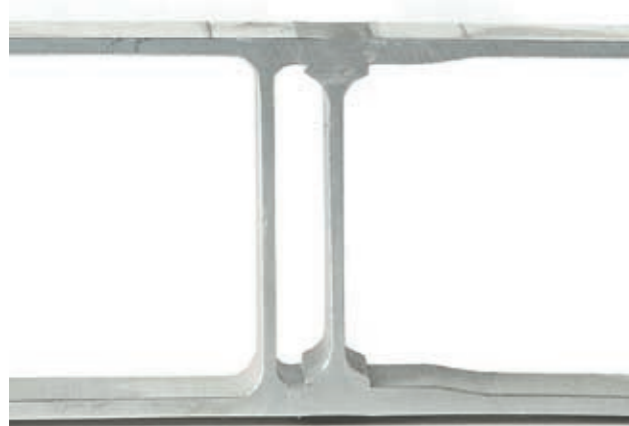
Figure 35. An extruded profile designed for friction stir welding.
