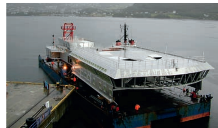
Figure 45. An over-hull structure at Marine Aluminium.
