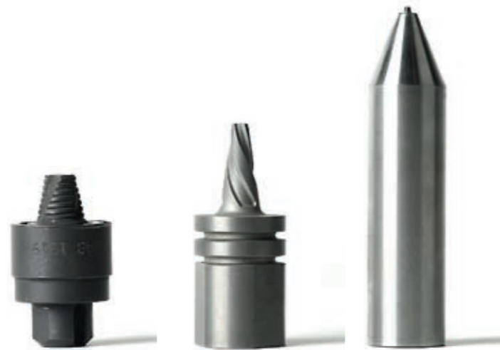
Figure 4. Pin-tool geometries for FSW tools.
