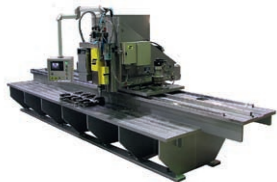
Figure 21. Modular LEGIO 5UT friction stir welding machine for flexible manufacturing. The working envelope of this particular equipment is 6000x500x300mm (x-, y-, z- axis). Delivered to KMT-teknikka OY, Finland, December 2003.
